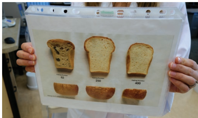
Cigi technicians measure "falling numbers" in flour samples: low falling numbers result from sprout damage.
